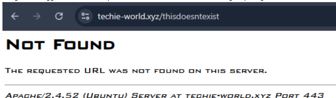
Figure 1 - Triggered an invalid request and received a verbose error message exposing internal server details.
